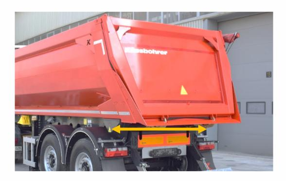
Specially designed wide tipping shaft provides better stability during your tipping operation by distributing load to a wider area to enhance operational safety.
