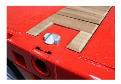
On the new series, new design **twistlocks** are available enabling to **attach** and **detach in seconds**. They are **retrofittable** for preferances after the purchase of the vehicle.
