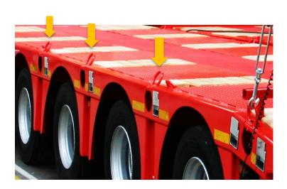
On the new series, new type forged lashing rings are available with increased capacity of 10 ton and 5 ton.
